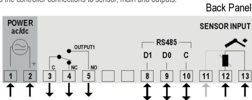
Pt100 with 3 conductors: Terminals 11, 12 and 13 must have the same wire resistance for proper cable length compensation. For 2 wire Pt100, short circuit terminals 12 and 13.
